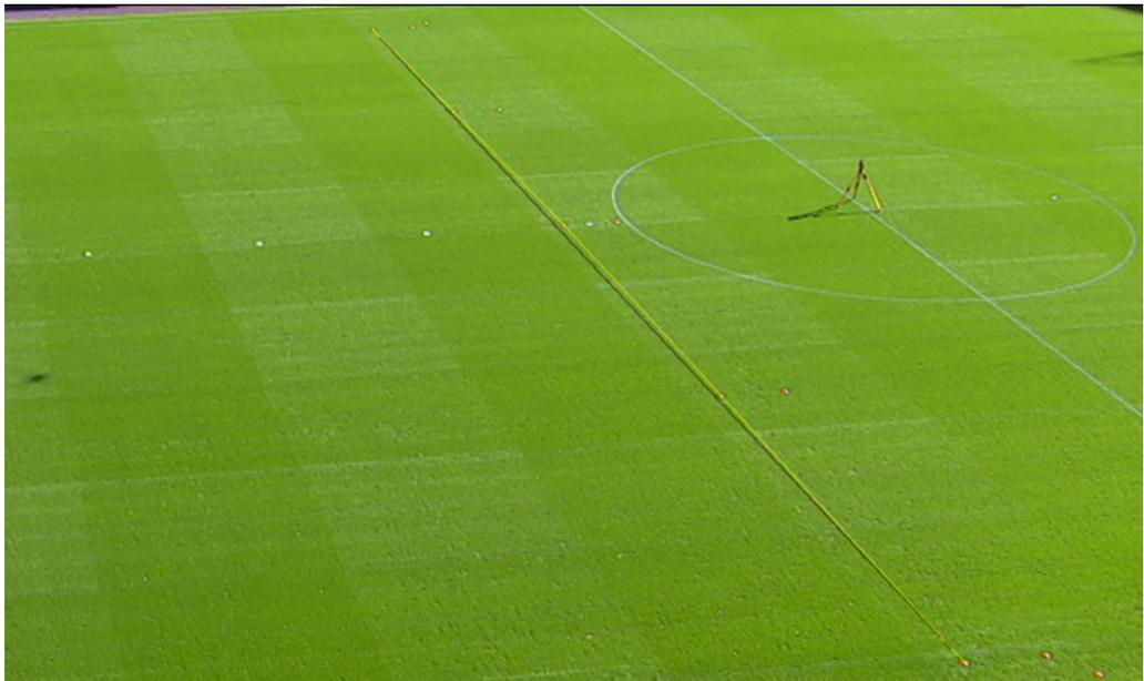
*Figure 3 - Representation of the external marker layout for Full Width scenarios - all virtual offside line leading edges must fall within the 500mm channel at each of the five zones (or trailing edge if applicable).*
