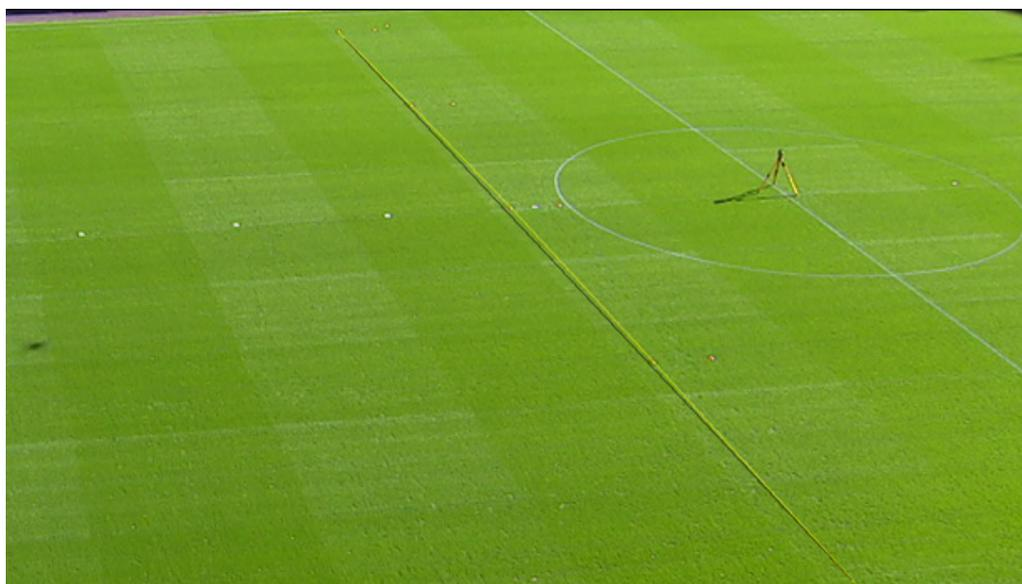
Figure 2 - Image from a previous testing set, showing a dynamic yellow line between the centre of the markers laid on the pitch showing that Ground Truth is accounted for at each zone, compared to a perfectly straight black line drawn between the widest markers.
