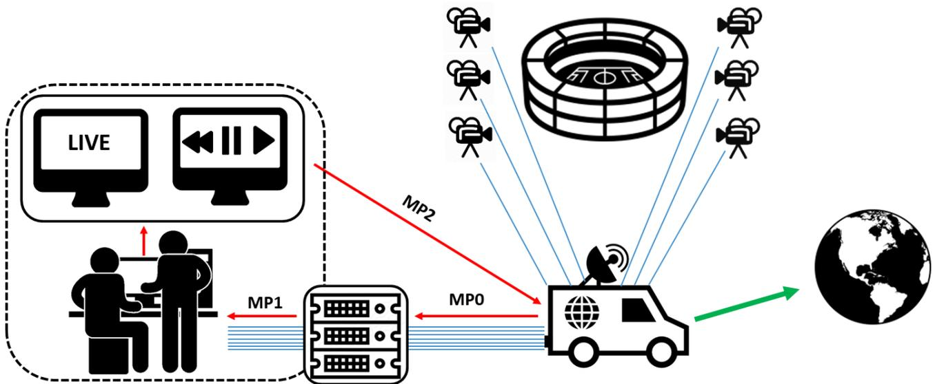
Figure 1: Schematic overview of the VAR setup. Three measurement points (MP) are indicated MP0, MP1 and MP2, for the evaluation of latency, synchronization and video quality.
