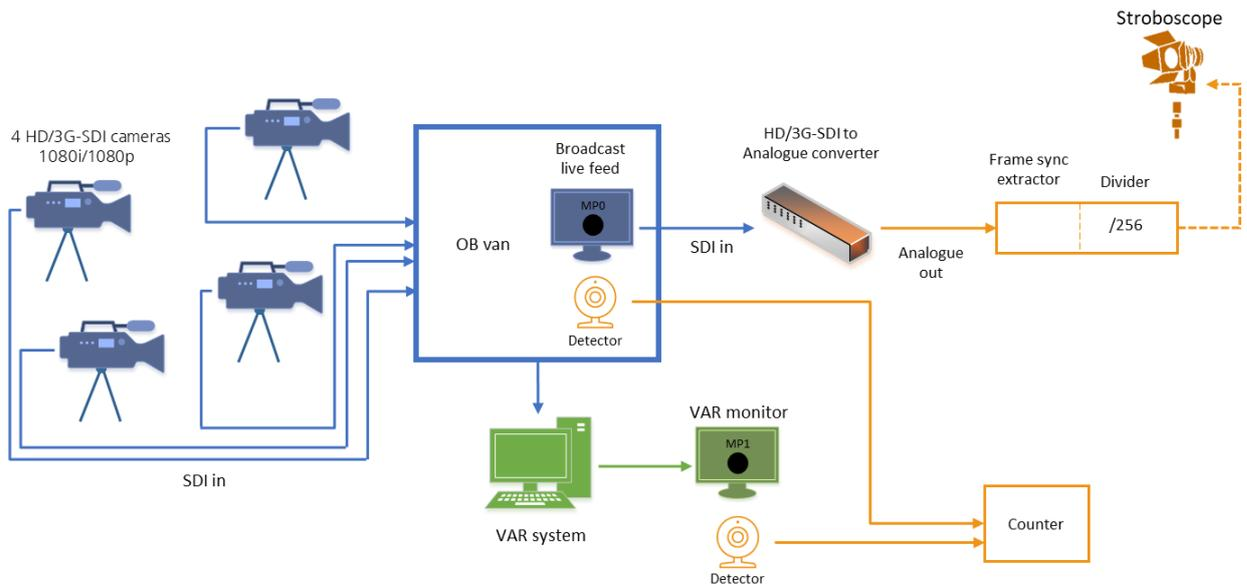
Figure 3: Latency test between the stroboscope flash in a broadcast feed and the VAR monitor.
