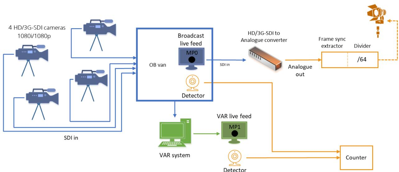
Figure 4: Latency test between stroboscope flashes and the VAR live feed.
