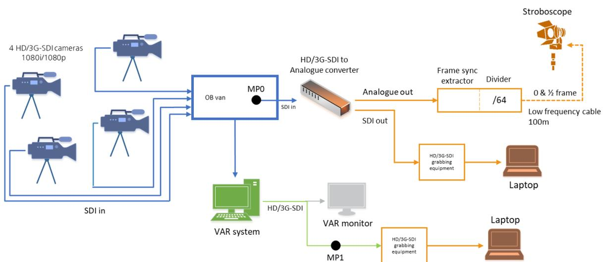
Figure 2: Synchronicity test at MPO and MP1.
