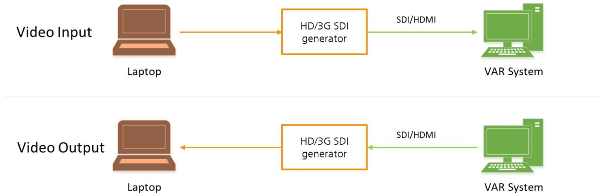
Figure 2: (left) Set-up for ingesting test video into a VAR system. (right) Set-up for recording test video from a VAR system.
